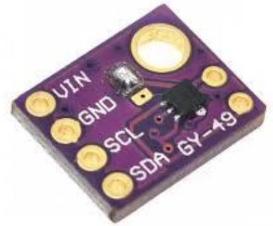
Within the light sensor, there is a sensing element that is sensitive to light in some manner. Usually, it is a type of diode or photoresistor which has a response to the light input that can be measured and transmitted effectively. This response is most commonly a voltage change across the discrete element that a controller can detect.
