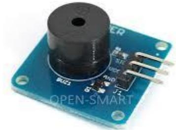
Piezoelectric speakers are often used in computers, alarms, timers, watches and other electronic devices to generate sound. They are also used as tweeters in less-expensive speaker systems, such as computer speakers and portable radios.
